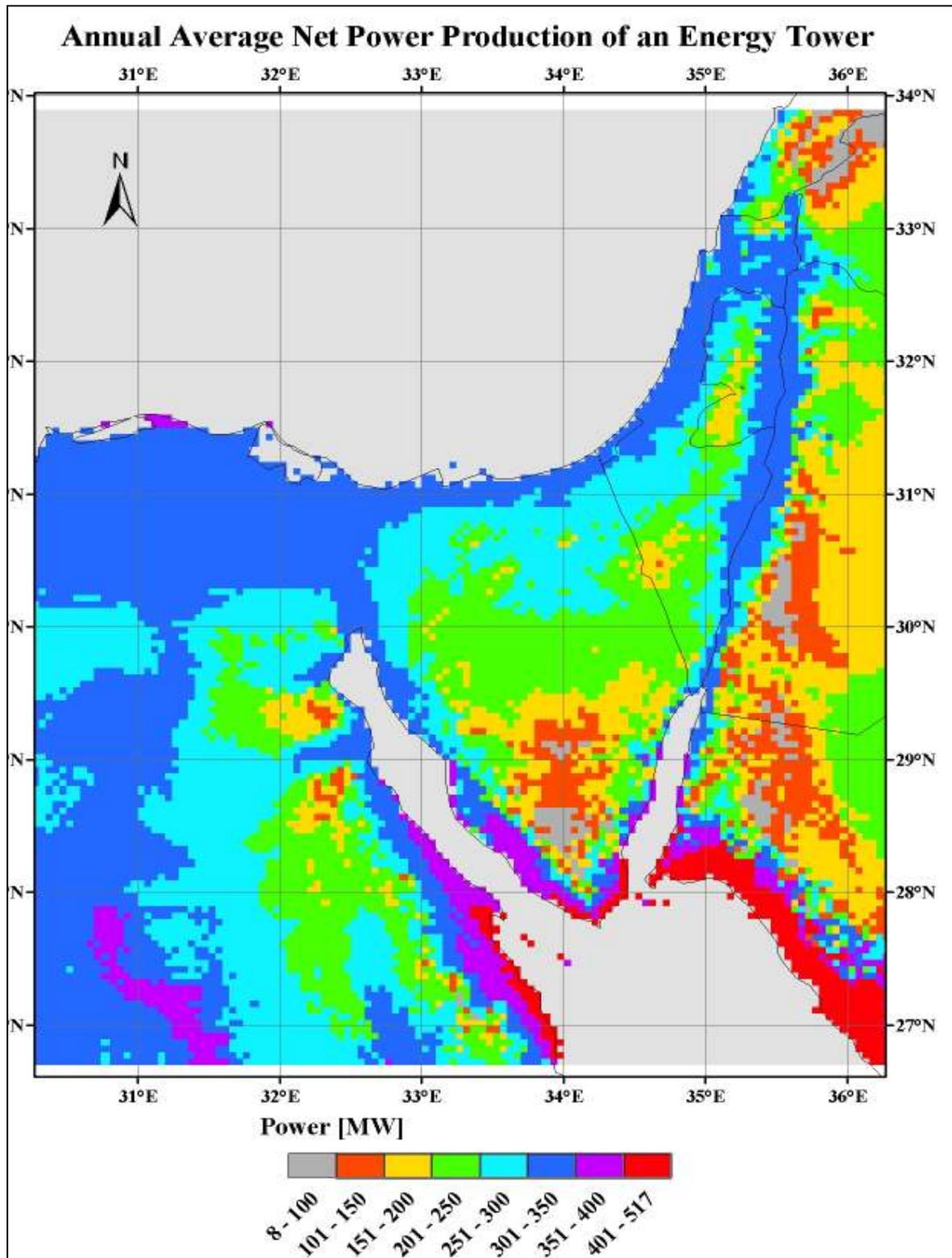
Figure 6 - Mapping of the net output from a standard design Tower in Israel and its neighbors (5x5 km area units)
