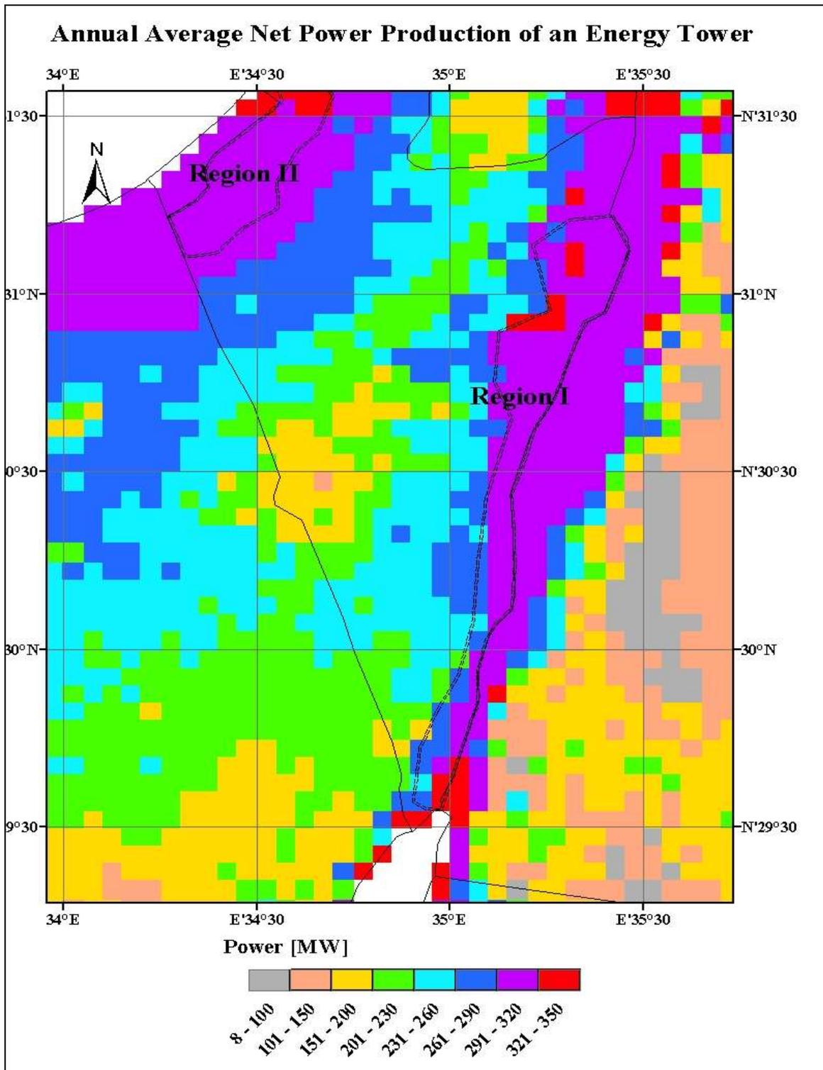
Figure 5 - Mapping of the net output from a standard design Tower in the South of Israel (5x5 km area units)
