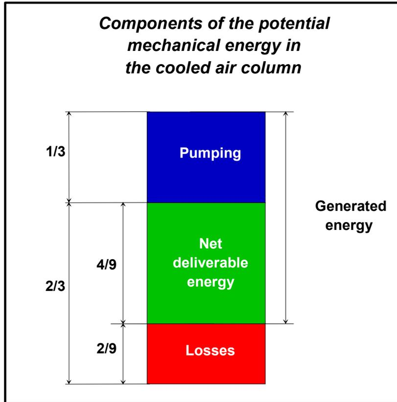
Figure 4 - Components of the mechanical energy (North of Eilat)
