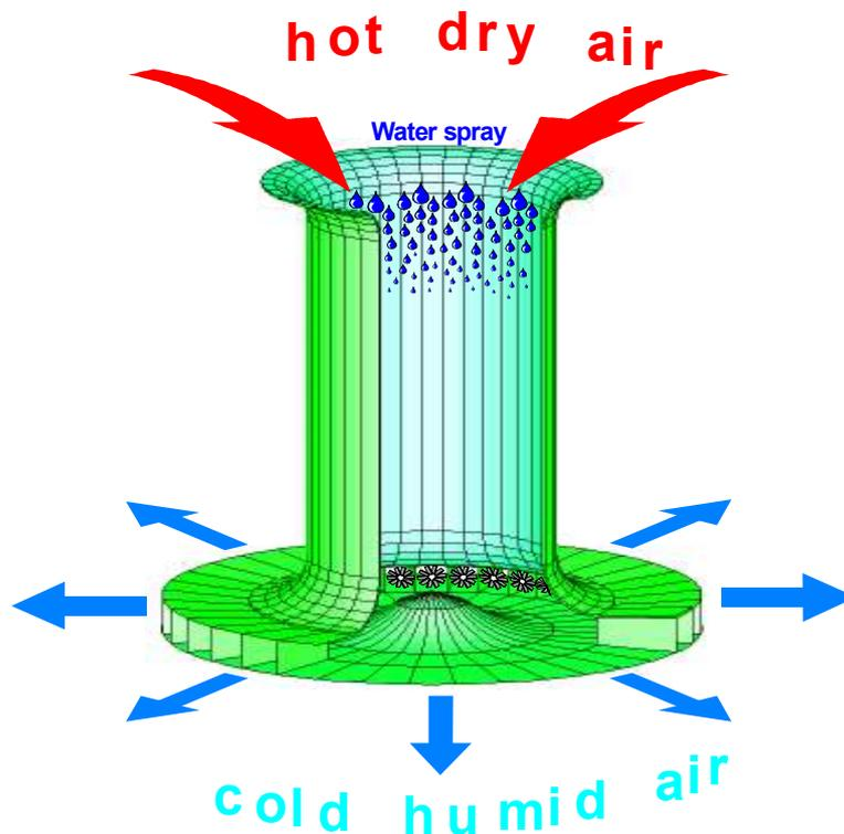
Figure 1 - The Energy Tower principle
